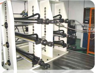
Seat and Seat Belt Anchorage Test
